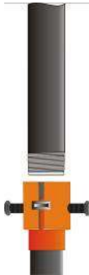
Figure 3 – Make-up with special bell guide
