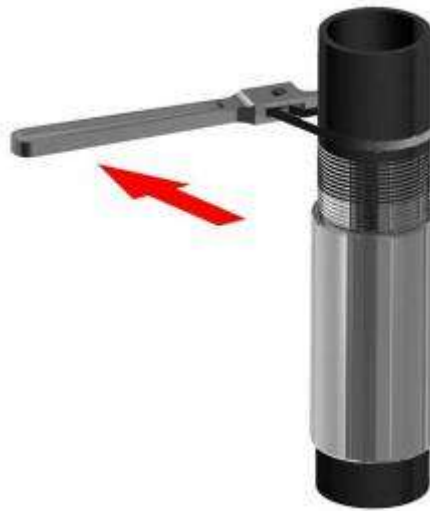
Figure 7 – Make-up start with strap tongs
