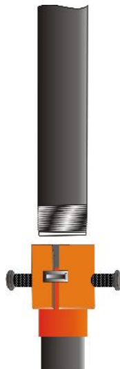
Figure 3 – Make-up with special bell guide
