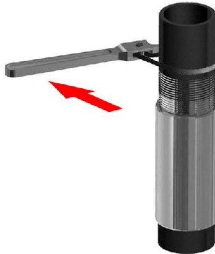
Figure 7 – Make-up start with strap tongs
