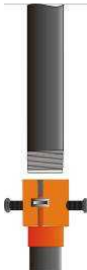
Figure 3 – Make-up with special bell guide
