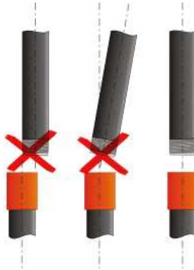
Figure 5 – Mechanical damage inspection
