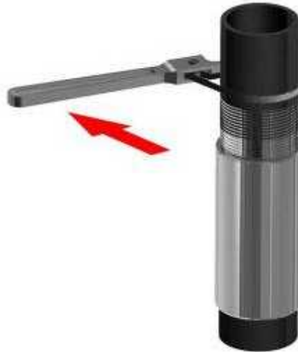
Figure 7 – Make-up start with strap tongs
