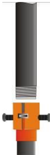
Figure 5 – Make-up with special bell guide
