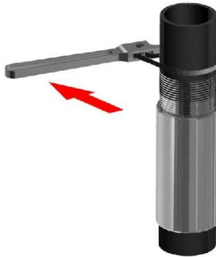
Figure 10 – Make-up start with strap tongs
